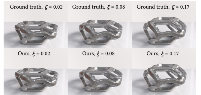
Figure 12: Our neural stress field can capture the hardening effect under different hardening coefficients
