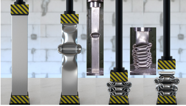
Fig. 24. Hydraulic Test on a Square Pipe. The crushing pattern matches the result of a real-world experiment [Youtube 2018].
